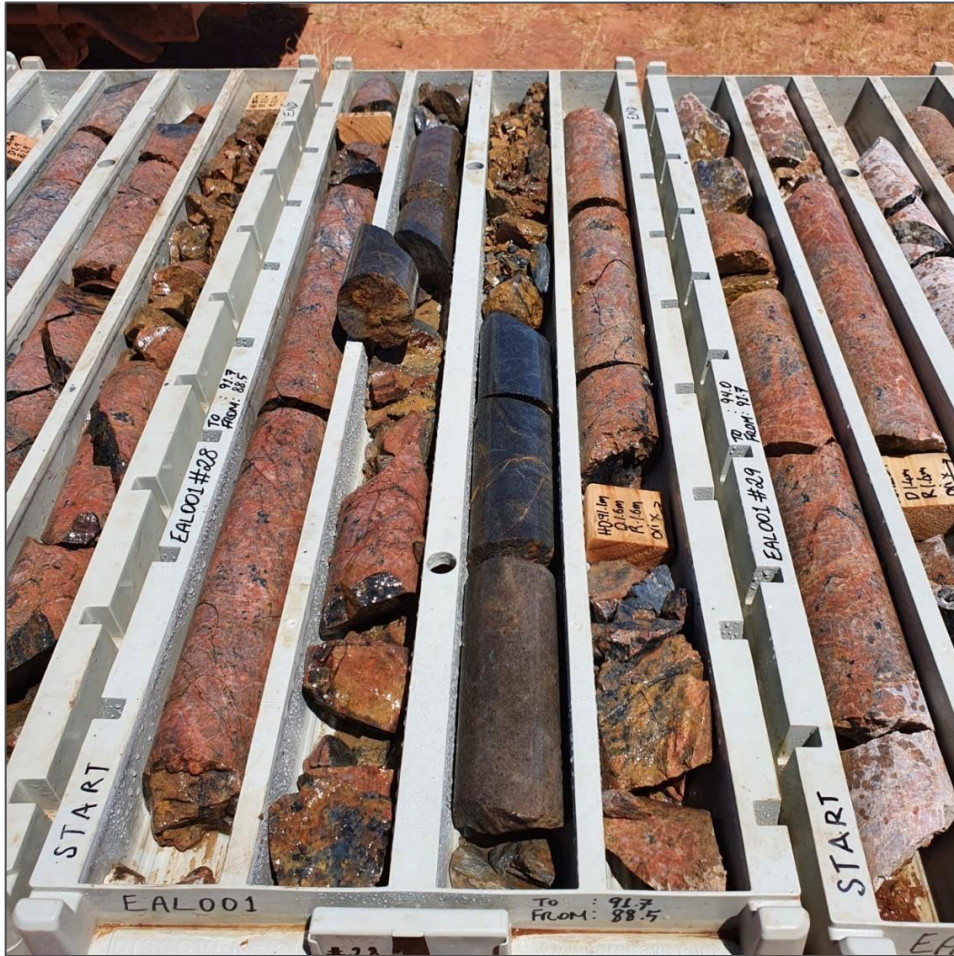
Hematite altered and fractured, coarse grained granitic rock with narrow mafic intrusive (88.5 - 91.7m)
