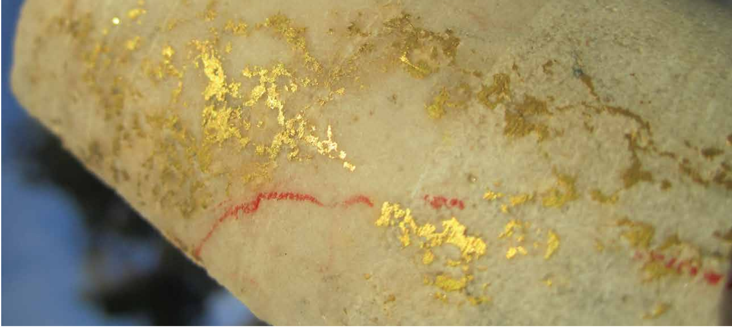
Fosterville: Lower Phoenix Fault - Eagle ore body, drill hole UDH1501: 12.5m @ 500.7 g/t Au (4.5m ETW)
